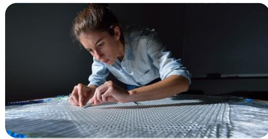
UM senior civil engineering student Rachel Tutor weaving quasi-three-dimensional S-Glass fibers for high velocity impact composites.
